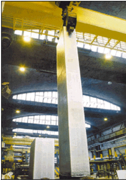
Figure 4: DC cast ingots
