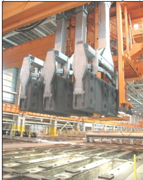
Figure 5: Carbon anodes after baking
