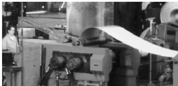
Not new either - twin roll casting ca 1956
